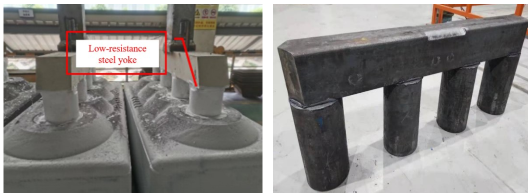
Figure 5. On-site test yokes. Left: low-resistance yoke, right: yoke with friction-welded stubs.
